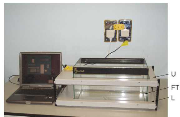
Fig. 1. Activity monitor used in the present study. U, upper level infrared beam source; L, lower level infrared beam source; FT, fish tank.
